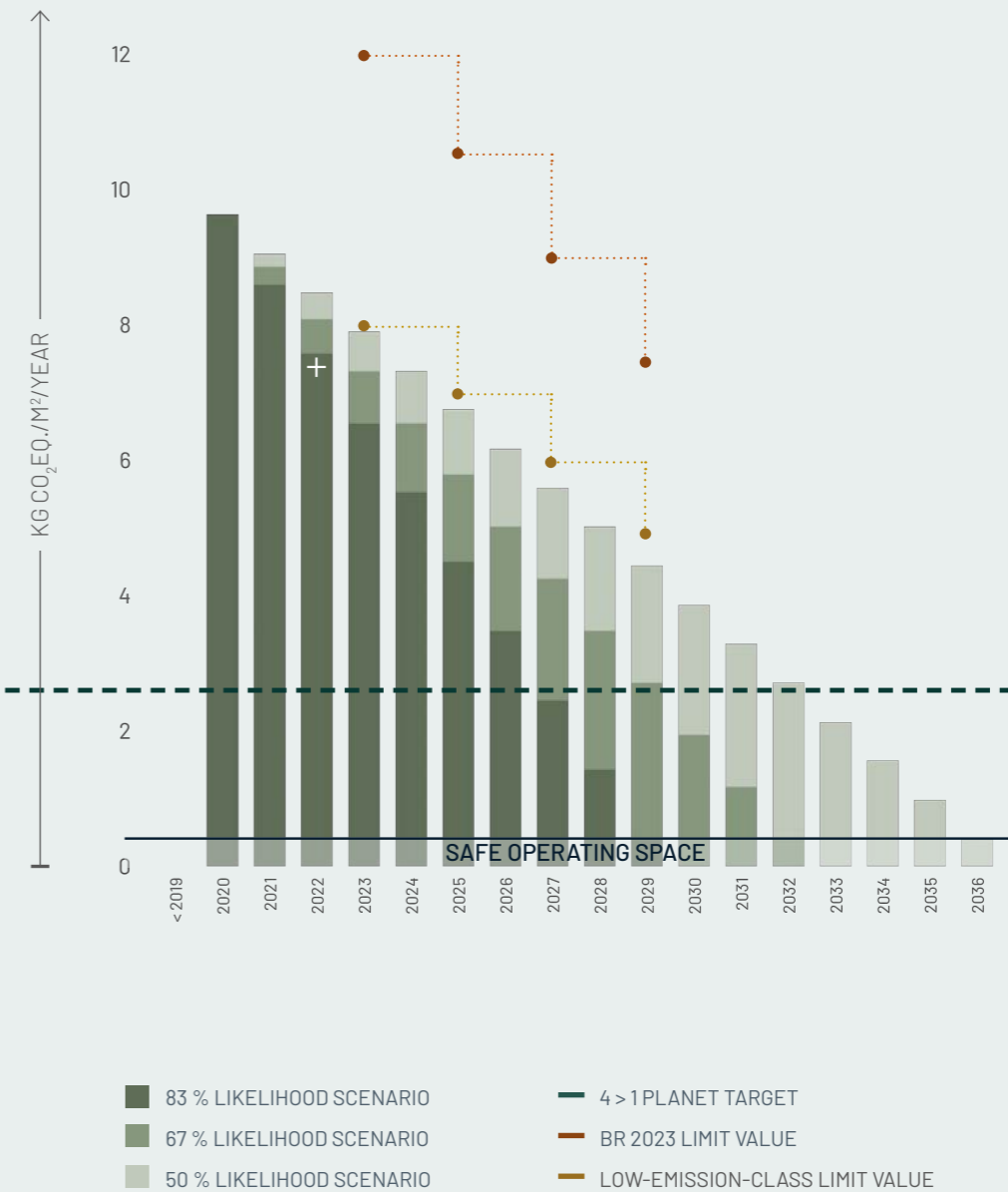
Figure E03.6: Reduction Roadmap The case study in relation to the Reduction Roadmap, limit values, the 4 to 1 planet goal of 2.5 kg CO 2 eq./m 2 /year, and the 'safe operating space'.
