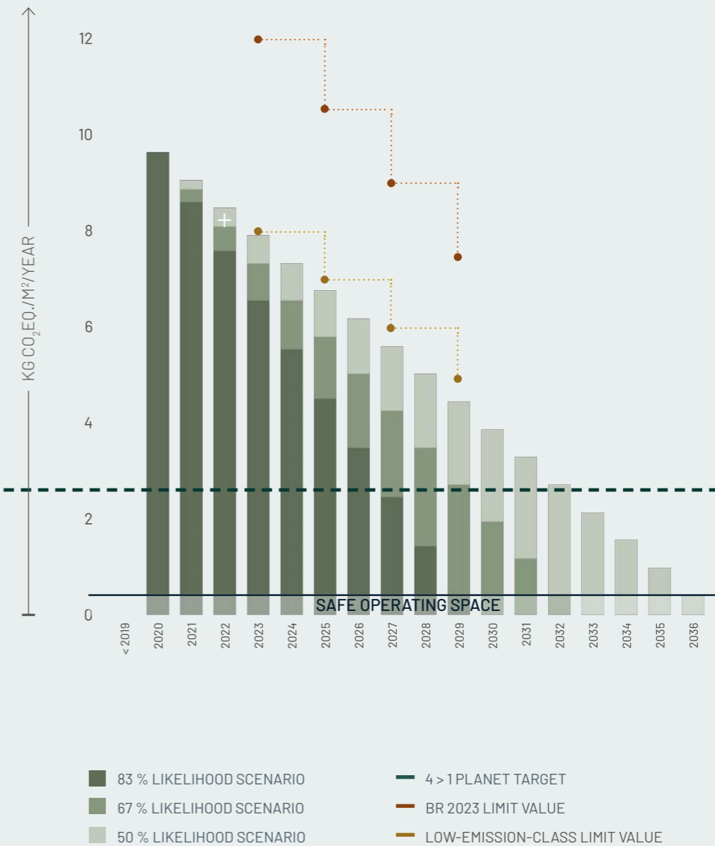
Figure ENF07.6: Reduction Roadmap The case study in relation to the Reduction Roadmap, limit values, the 4 to 1 planet goal of 2.5 kg CO 2 eq./m 2 /year, and the 'safe operating space'.
