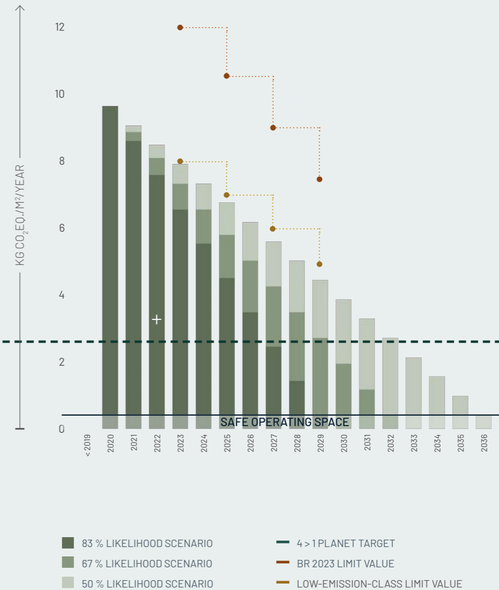
Figure E06.6: Reduction Roadmap The case study in relation to the Reduction Roadmap, limit values, the 4 to 1 planet goal of 2.5 kg CO 2 eq./m 2 /year, and the 'safe operating space'.
