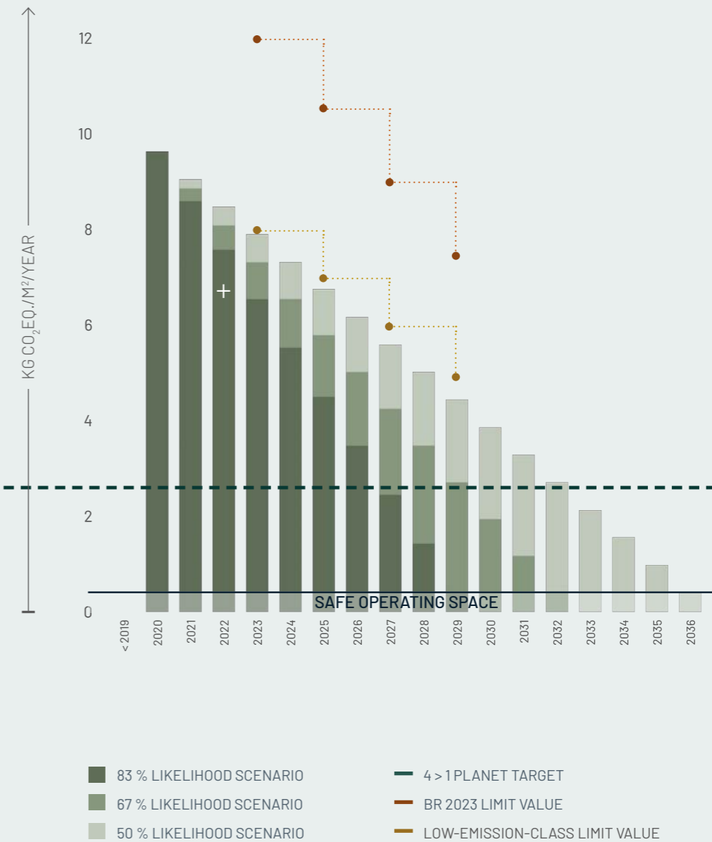
Figure R03.6: Reduction Roadmap The case study in relation to the Reduction Roadmap, limit values, the 4 to 1 planet goal of 2.5 kg CO 2 eq./m 2 /year, and the 'safe operating space'.
