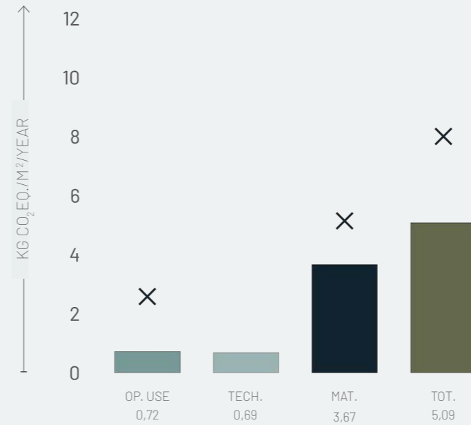
Figure E02.1: Emissions of kg CO 2 eq./m 2 /year The bars show the building's environmental impact. Crosses indicate the highest result for operational use, materials, and total emissions of kg CO 2 eq./m 2 /year in multi-storey housing in the case collection.
