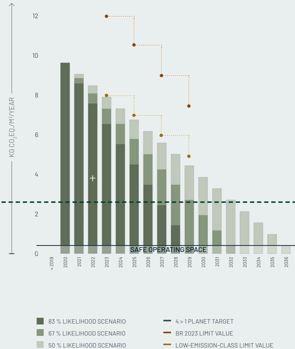
Figure ENF01.6: Reduction Roadmap The case study in relation to the Reduction Roadmap, limit values, the 4 to 1 planet goal of 2.5 kg CO 2 eq./m 2 /year, and the 'safe operating space'.
