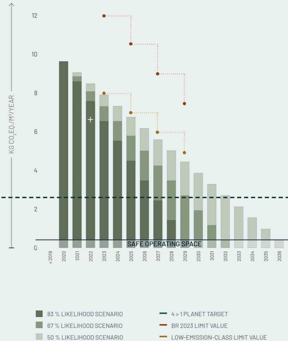
Figure ENF09.6: Reduction Roadmap The case study in relation to the Reduction Roadmap, limit values, the 4 to 1 planet goal of 2.5 kg CO 2 eq./m 2 /year, and the 'safe operating space'.
