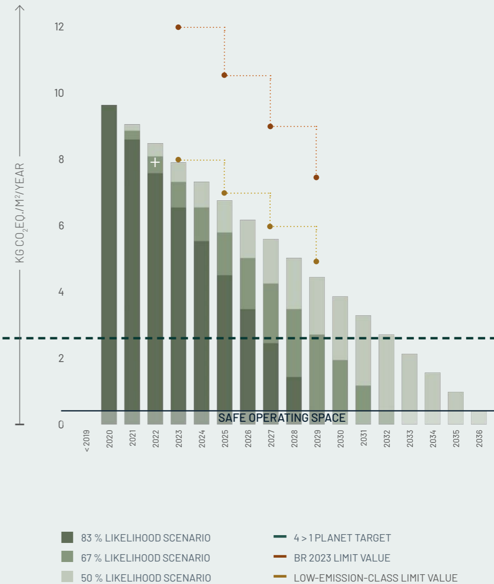
Figure E01.6: Reduction Roadmap The case study in relation to the Reduction Roadmap, limit values, the 4 to 1 planet goal of 2.5 kg CO 2 eq./m 2 /year, and the 'safe operating space'.
