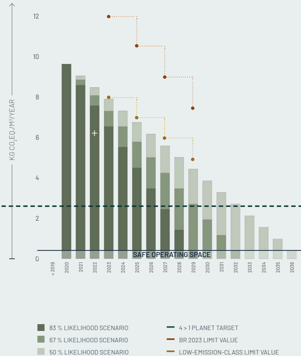
Figure ENF02.6: Reduction Roadmap The case study in relation to the Reduction Roadmap, limit values, the 4 to 1 planet goal of 2.5 kg CO 2 eq./m 2 /year, and the 'safe operating space'.
