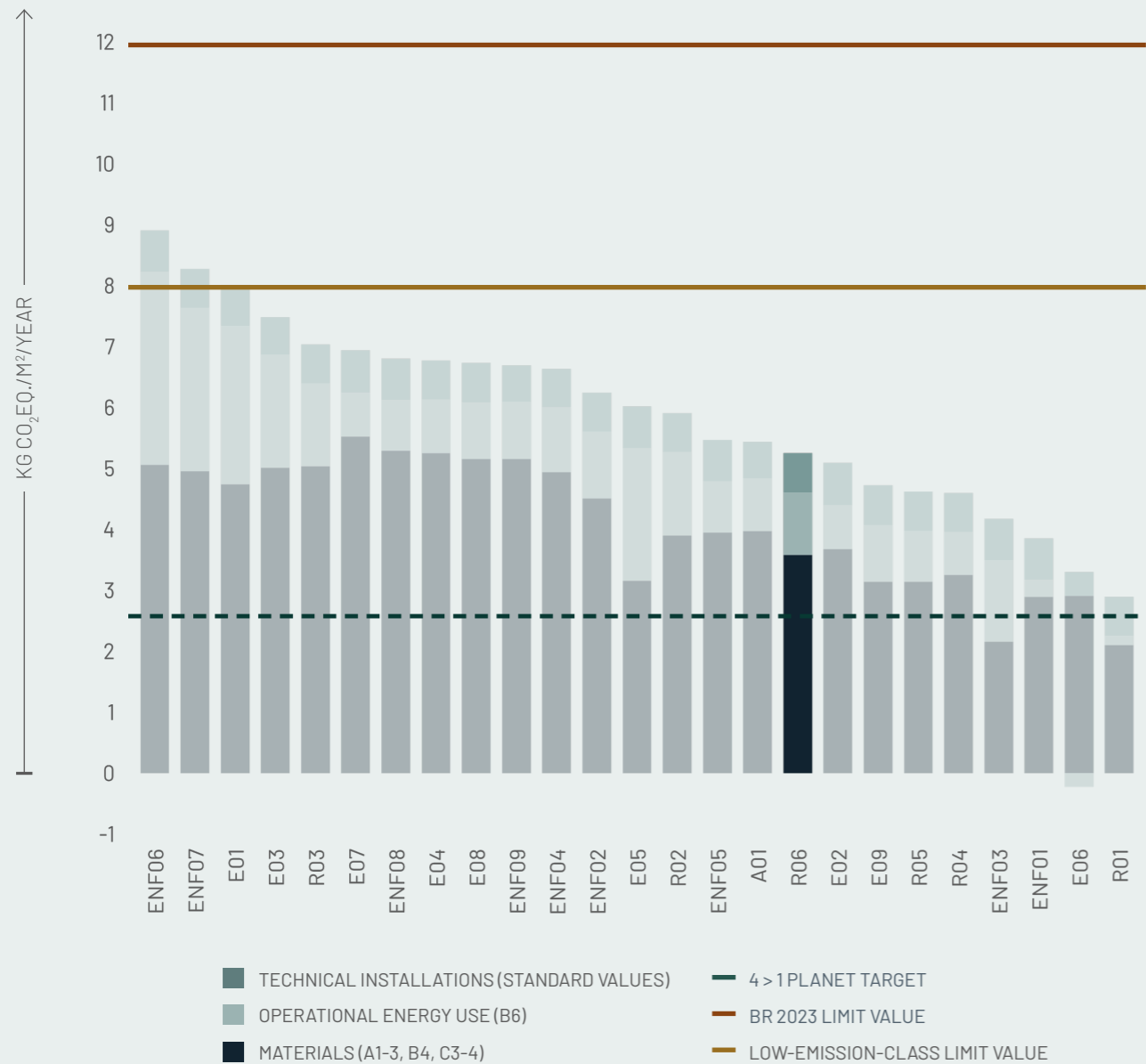
Figure R06.5: Housing case studies The vertical axis shows the emission of CO 2 eq./m 2 /year. The horizontal axis shows the 25 best practice cases.
