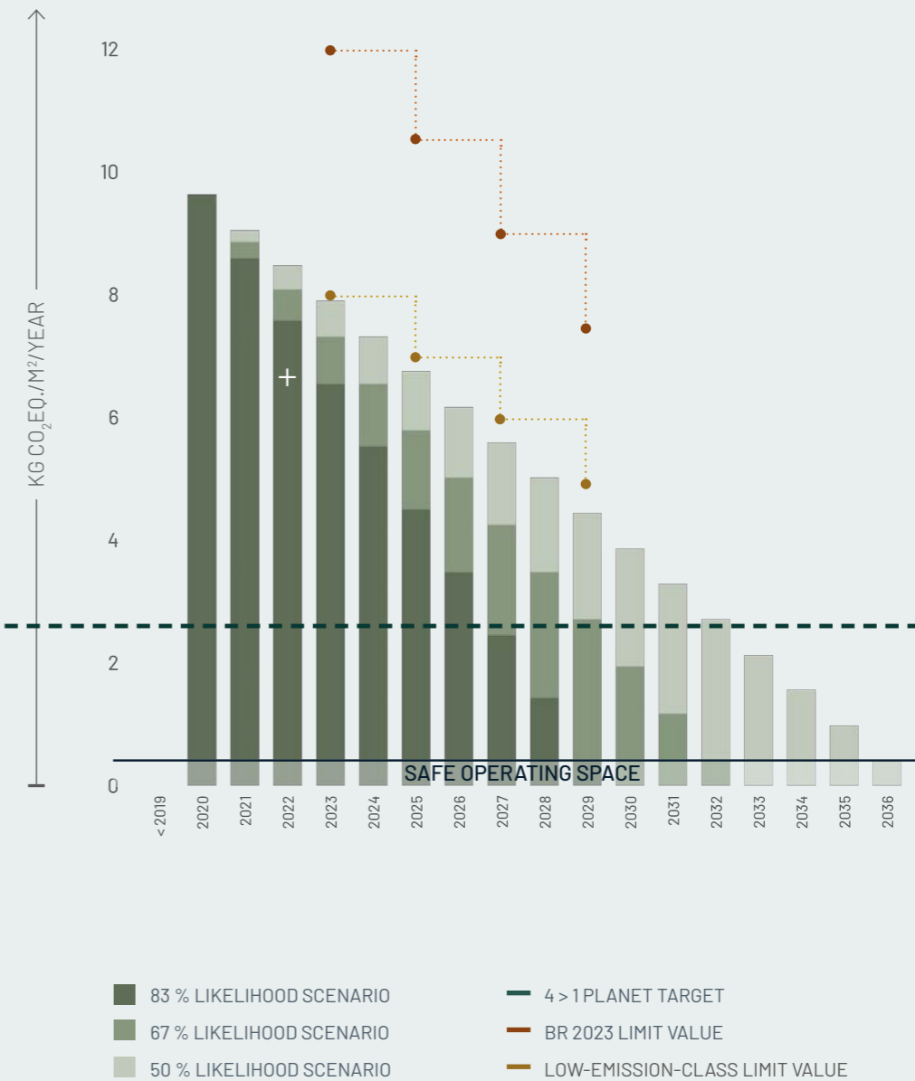
Figure E08.6: Reduction Roadmap The case study in relation to the Reduction Roadmap, limit values, the 4 to 1 planet goal of 2.5 kg CO 2 eq./m 2 /year, and the 'safe operating space'.
