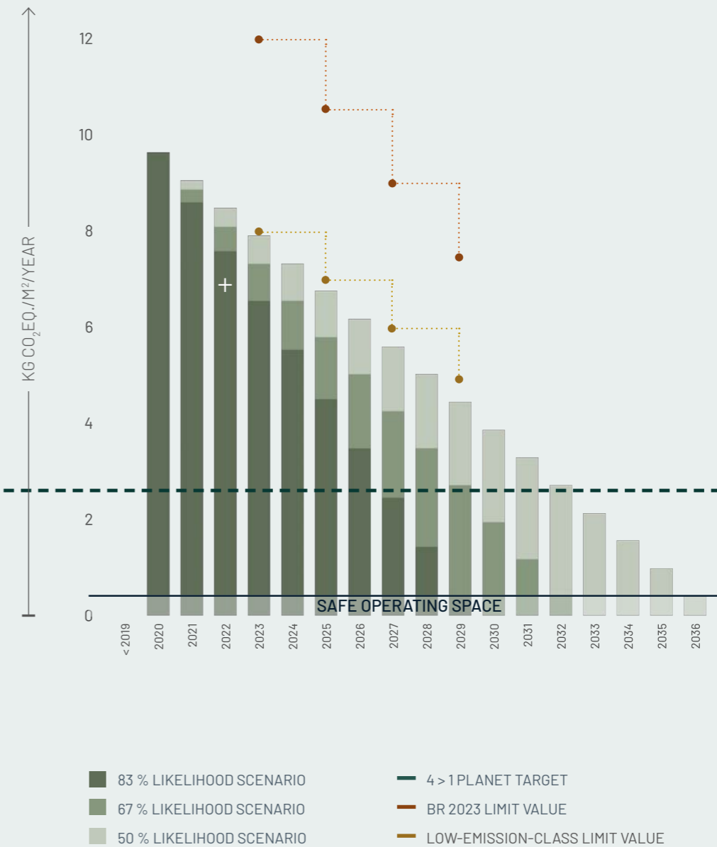
Figure E07.6: Reduction Roadmap The case study in relation to the Reduction Roadmap, limit values, the 4 to 1 planet goal of 2.5 kg CO 2 eq./m 2 /year, and the 'safe operating space'.
